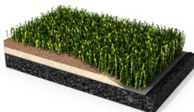
**FIH Multi-sport** category surfaces are surfaces designed for a number of sports including hockey. Primarily based on surfaces with longer piles that are infilled with rubber and sand (often described as third generation or 3G surfaces), the category also includes some forms of sand filled surfaces, needle-punch textile surfaces, etc.
